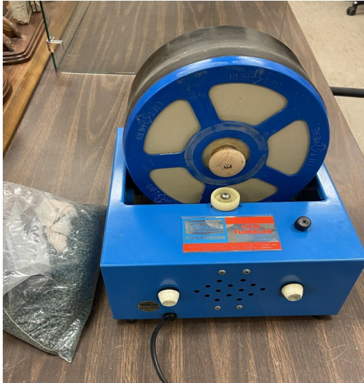
Sears Rock Tumbler: Model: 861.14171 Capacity: 8 pounds ? Drum Dimensions: 4"H x 8.3"Dia.
